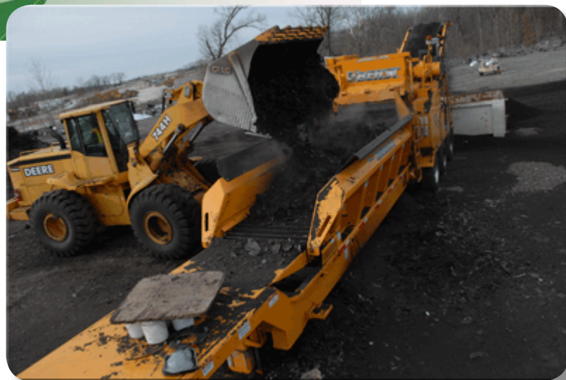
Shingles are ground up and processed.
