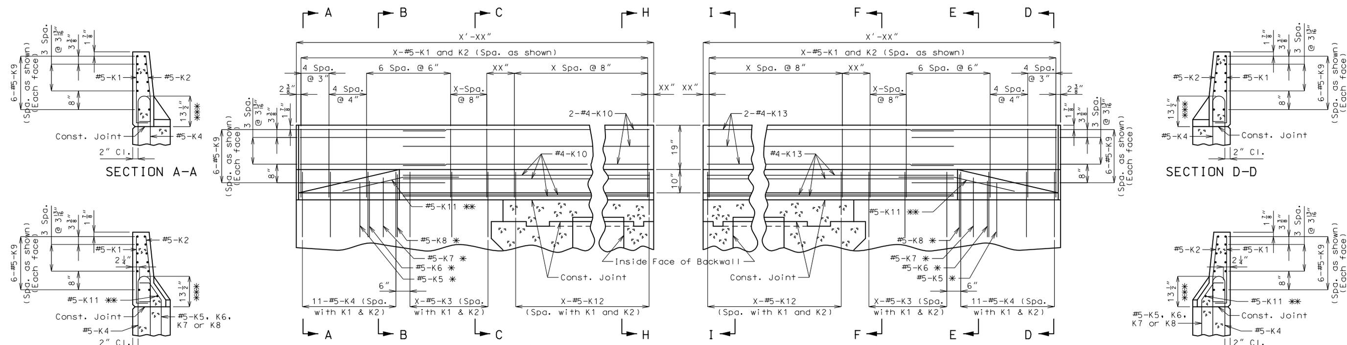
**ELEVATION** \* Spaced with #5-K4 bars and embed 27" into end bent.
