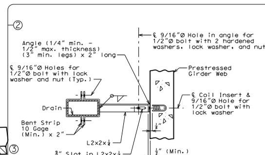
PART SECTION SHOWING BRACKET ASSEMBLY
