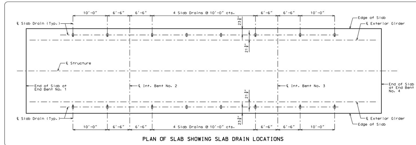
PLAN OF SLAB SHOWING SLAB DRAIN LOCATIONS
