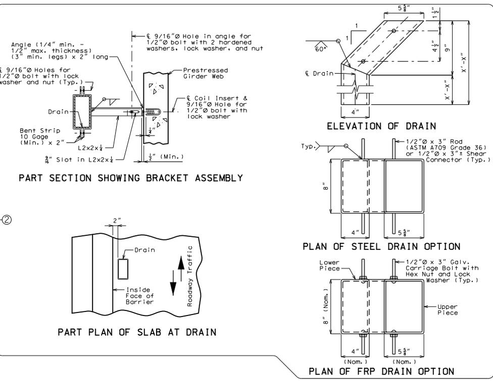
PART SECTION SHOWING BRACKET ASSEMBLY
