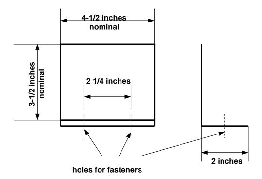
Delineator to have a minimum of 2 primary holes spaced as shown above. If additional holes are provided they shall be "in line" parallel to the face of the delineator.
