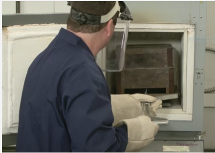
Determining the Asphalt Binder Content of Asphalt Mixtures by the Ignition Method 31
