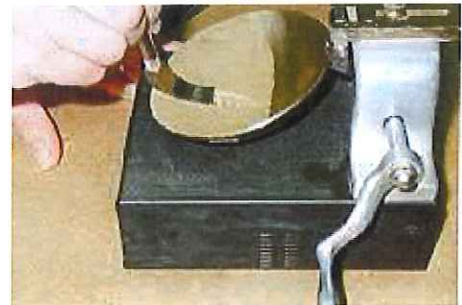
Applying blows by turning the handle
