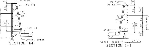
ALTERNATE DETAILS FOR SKEWED BRIDGES REQUIRING K3 BARS
