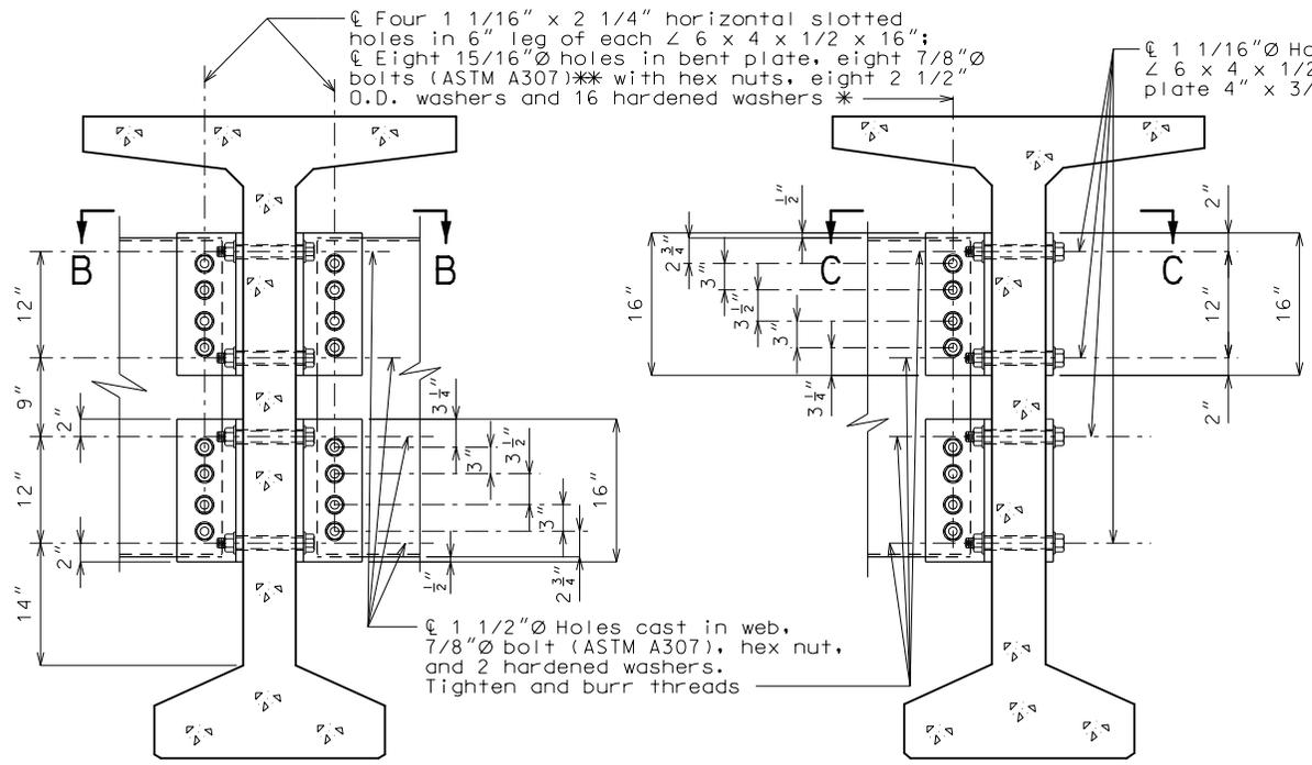
SECTION THRU INT. GIRDER AT DIAPHRAGM
