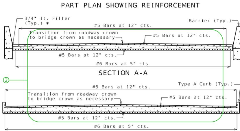
With the approval of the engineer, the contractor may crown the bottom of the approach slab to match the crown of the roadway surface.
