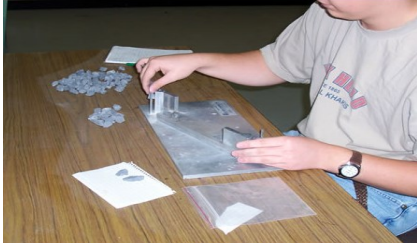
Flat Particles, Elongated Particles, or Flat and Elongated Particles in Coarse Aggregate
