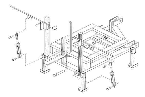
3 POINT HITCH CARRIAGE FOR ADAPTABLE SLOPE TRACTOR SPRAYER
