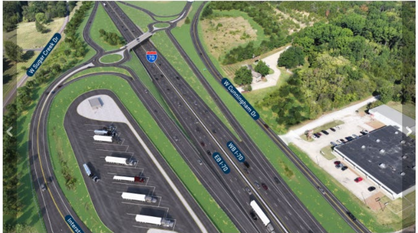
Future improvements at I-70 and Midway. Improvements include new dogbone interchange, relocated eastbound I-70 on ramp, and new truck parking facilities.
